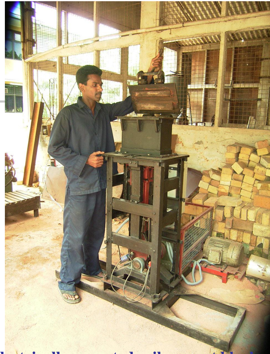
Electrically operated soil-cement block making machine. Capacity – 1500 blocks per day
