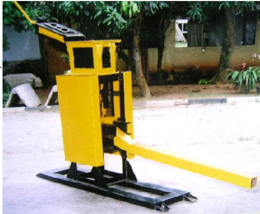
Manually operated soil-cement block making machine. Capacity 300-400 blocks per day
