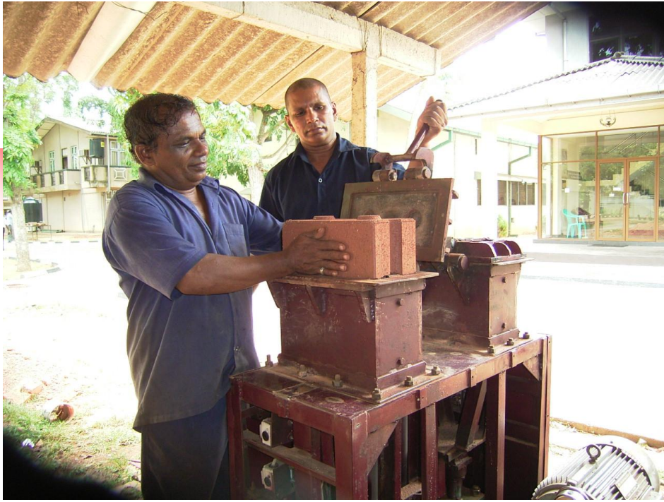
Soil cement blocks making machine operated by a Hydraulic system Capacity – about 1500 blocks per day
