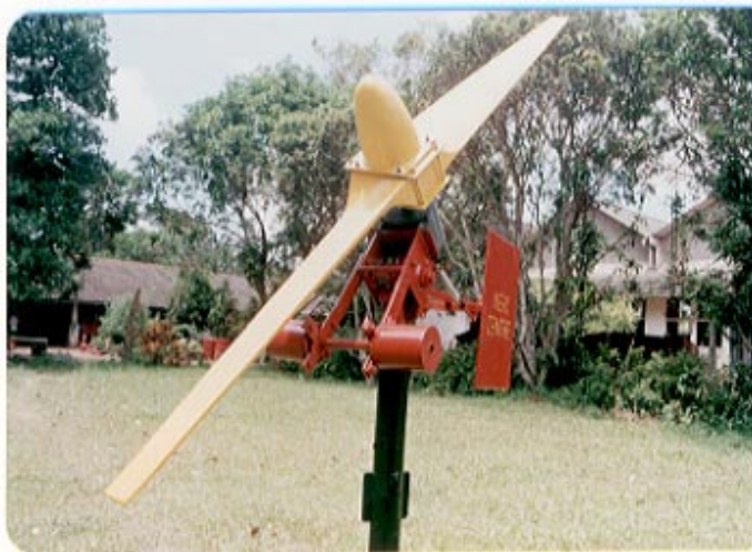
Wind rotor tilt up ward, when wind speed goes beyond the rated wind speed.
